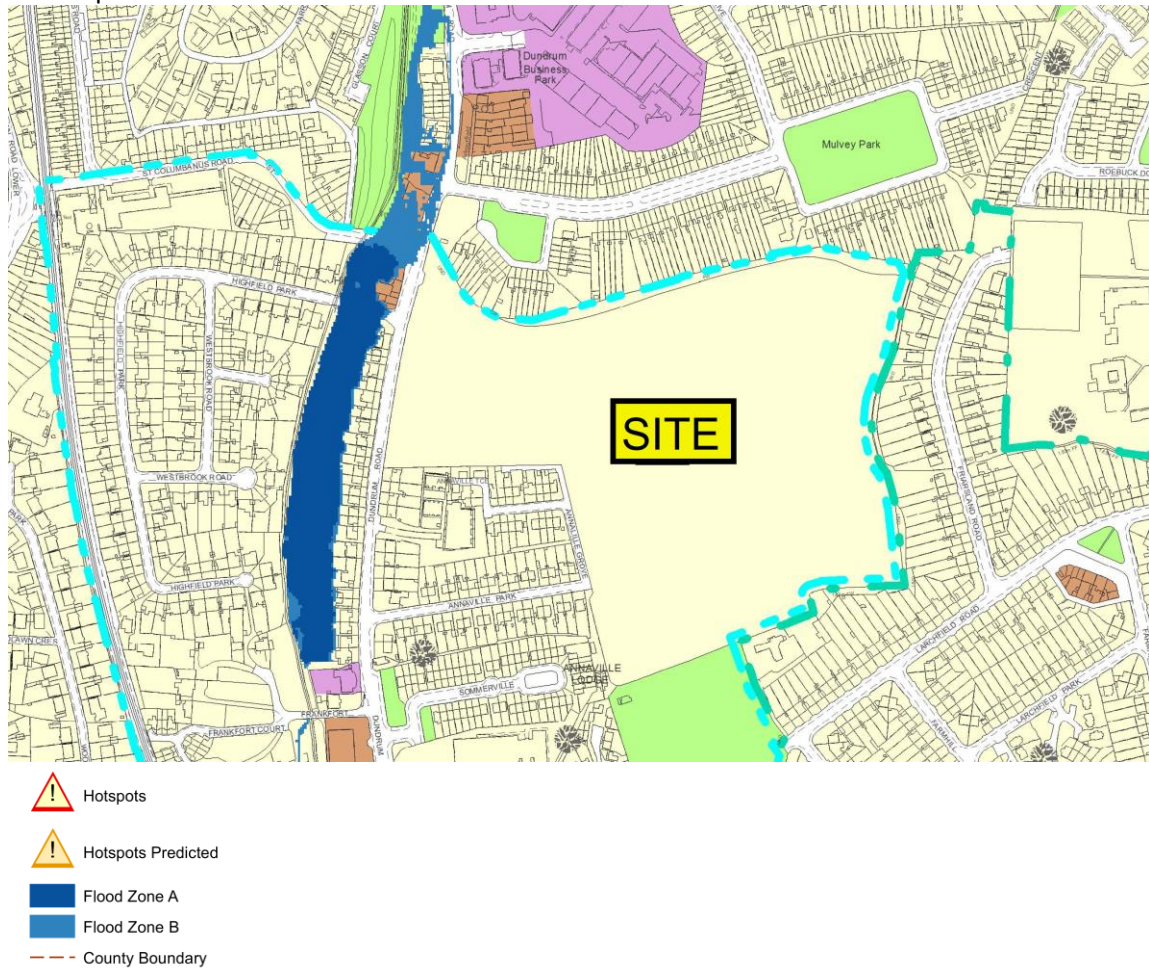
Fig 3.1 Extract from DL RCC Flood Zone Map 1. The site lies outside of the River Slane flood zones which are west of the Dundrum Road.
