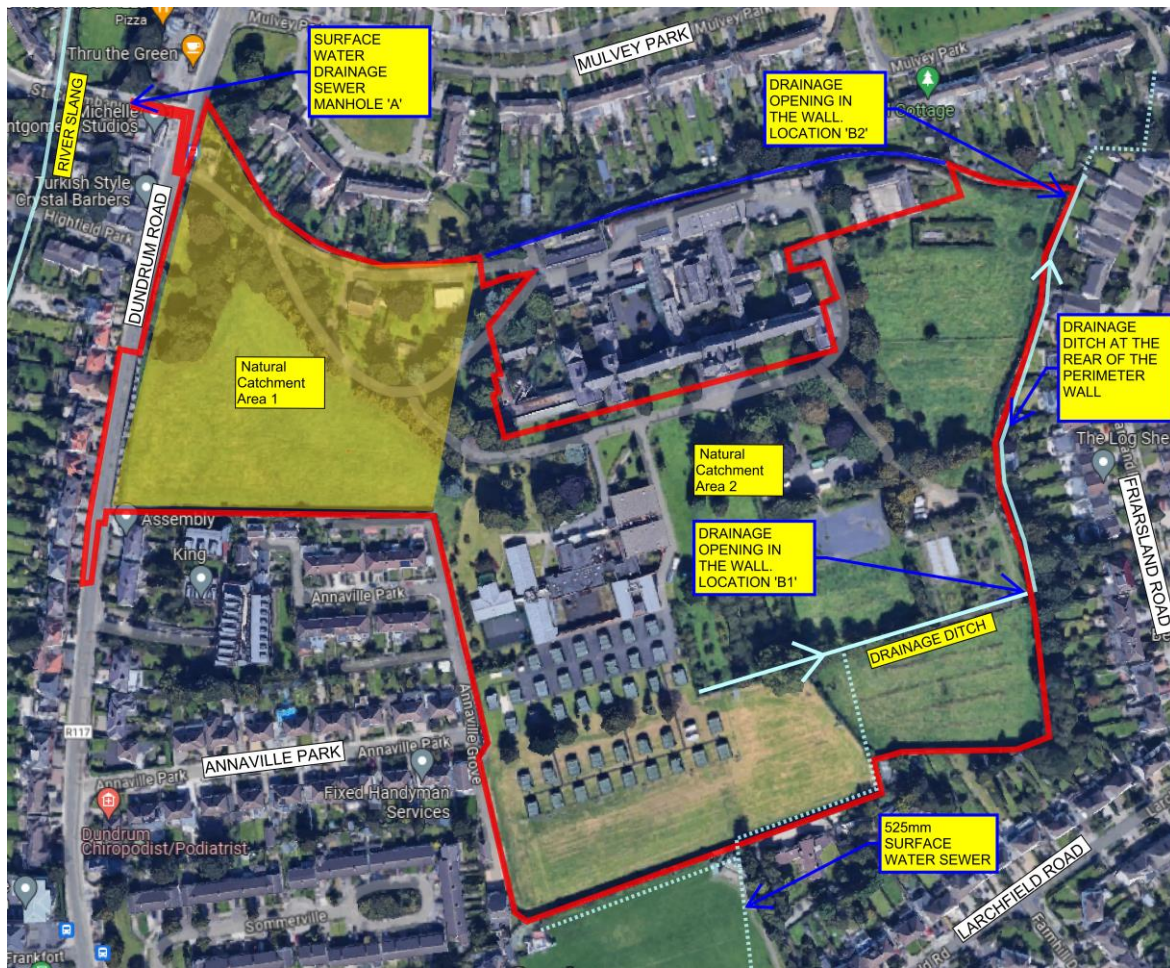
Fig 3.2. Aerial View of the Approximate Natural Catchment Areas of the Existing Site. Catchment 2 is in the unshaded area.
